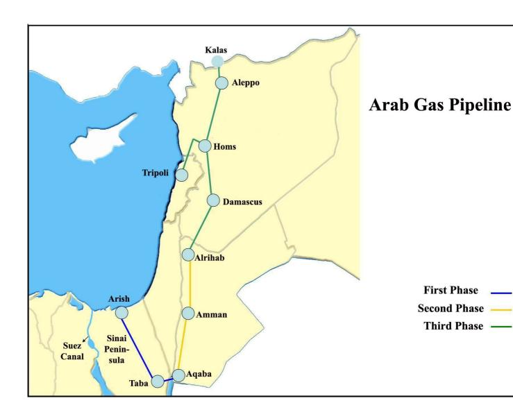
The pipeline would be built in three phases: first from Arish to Taba and Aqaba, then from Aqaba to Alrihab in Jordan, and finally from Alrihab to Kalas (or Kilis) in Turkey.
